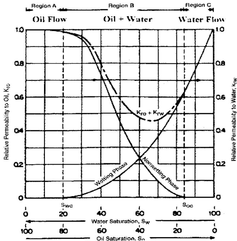
Figure 2.2: Typical two-phase (water-oil) flow behaviour.
