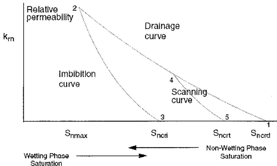
Figure 2.4: A typical pair of relative permeability curves for a non-wetting phase
