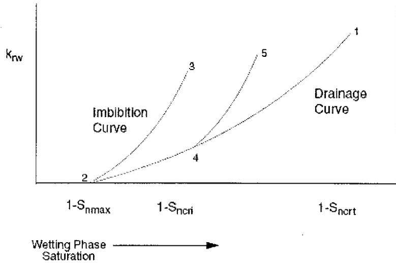
Figure 2.5: A typical pair of relative permeability curves for a wetting phase
