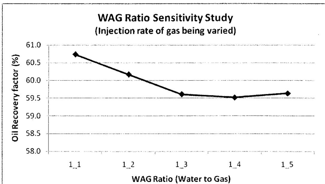
Figure 4.6: Oil Recovery rate for WAG Ratio Sensitivity Study
