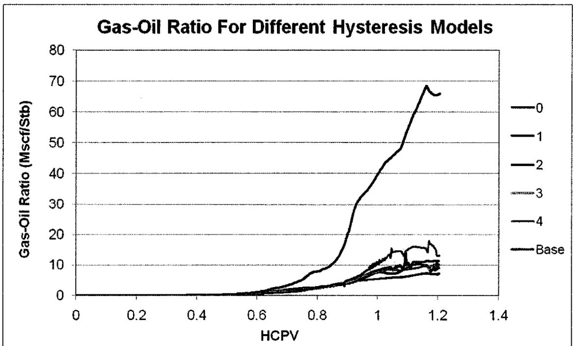
Figure 4.12: Gas-Oil Ratio for Different Hysteresis Models
