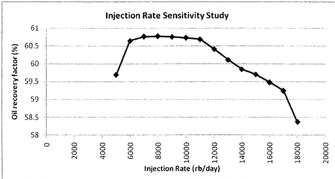
Figure 4.2: Oil Recovery Rate for Injection Rate Sensitivity Study
