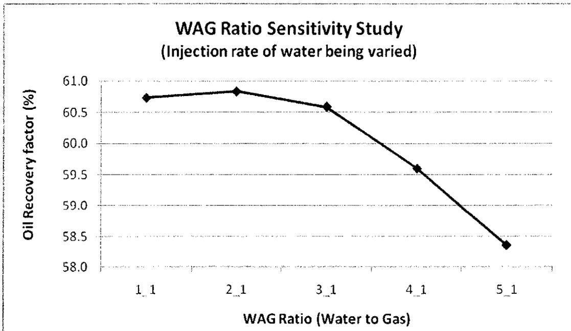
Figure 4.8: Oil Recovery rate for WAG Ratio Sensitivity Study (Injection rate of water being varied)
