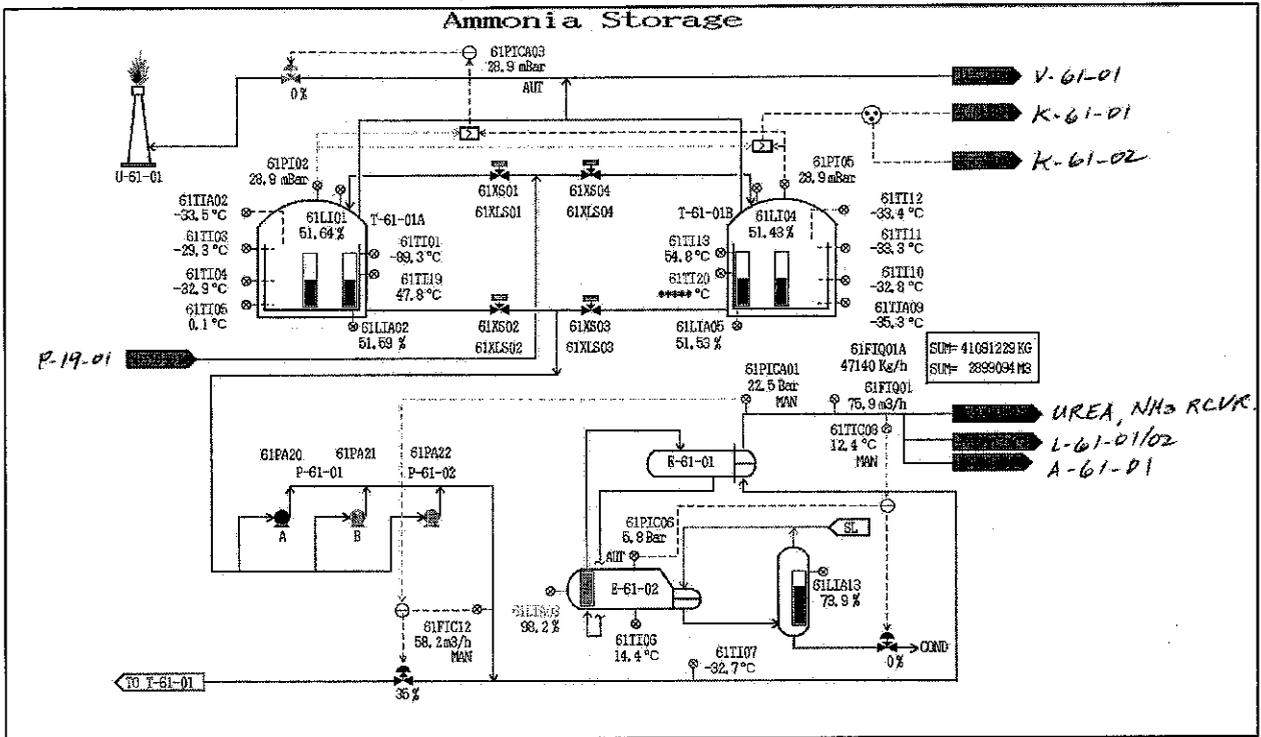
Figure AIII: Ammonia Storage Tank Location in Distributed Control System (DCS)
