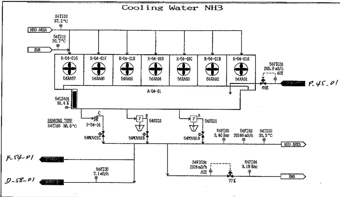
Figure AIV: Ammonia Cooling Tower Location in Distributed Control System (DCS)
