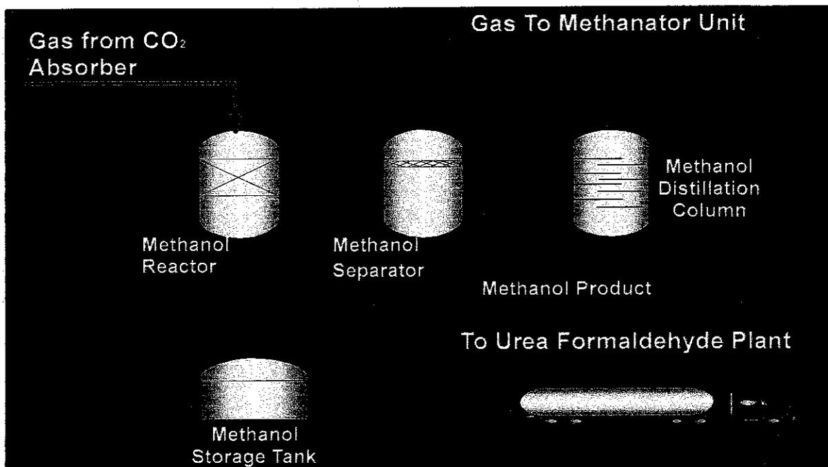
Figure AII: General Process and Area of Methanol Unit
