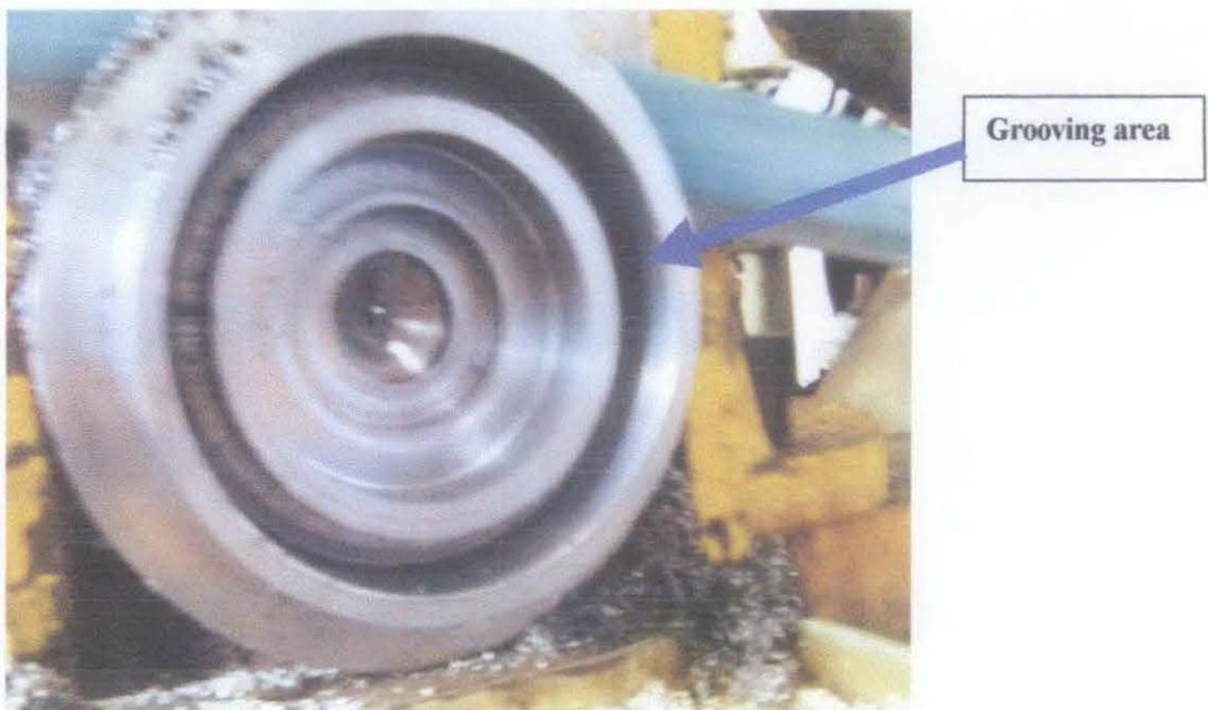
Figure 4.15: Grooving area in the stationary joint
