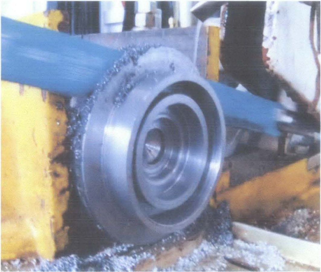
Figure 4.12: Parting process of the stationary joint using Linear Hack Saw machine
