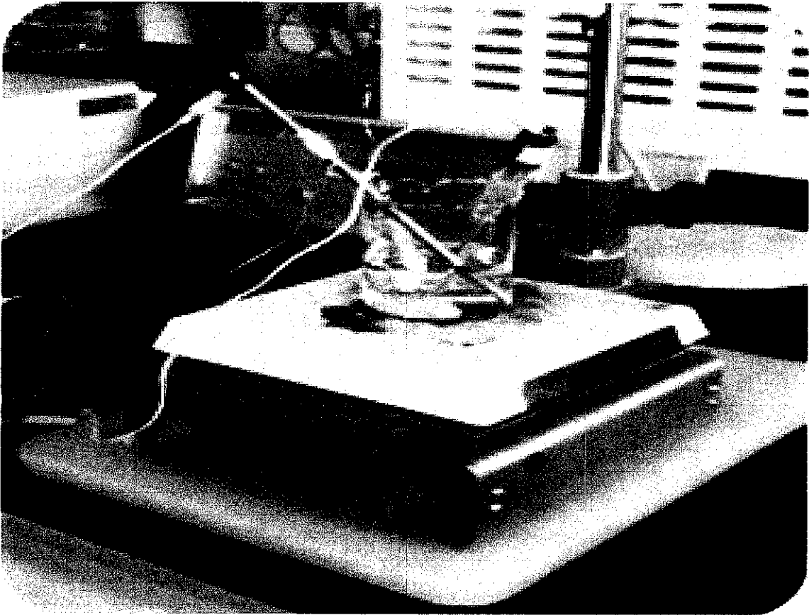
Figure 11: The electrode is tested using anodic stripping voltammetry (ASV)
