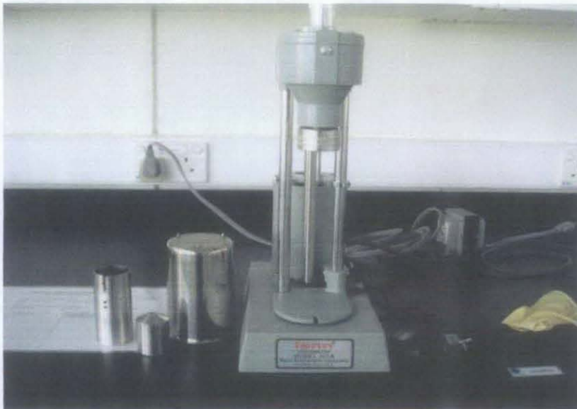
Figure-8' Viscometer and Controlled Cup (API Standard -13B)
