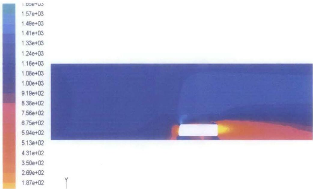
**Figure 4.4a: Spoiler model B ( $15^\circ$ ) dynamic pressure contour at 45 m/s.**
