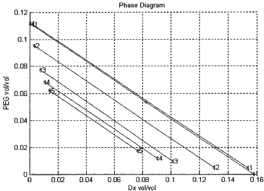
**Figure 8:** Phase diagrams of PEG 8000 - Dextran 75 at 23°C [30].
