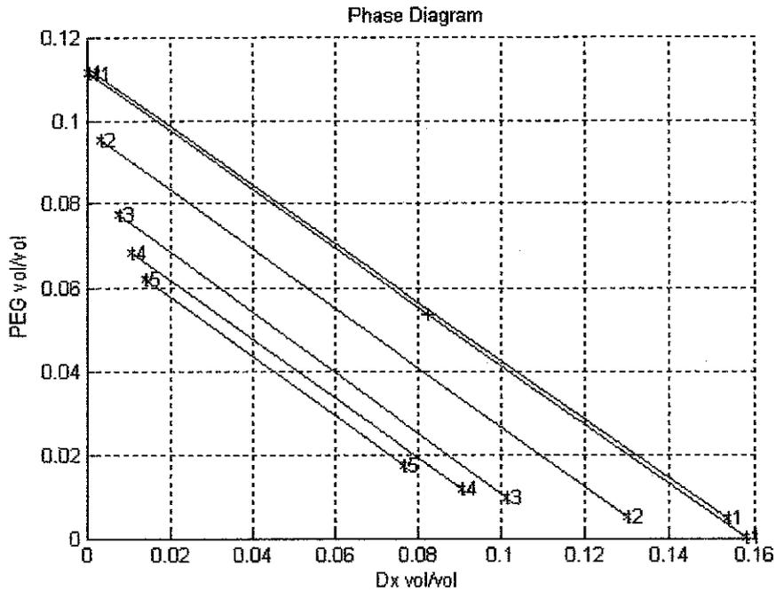
**Figure 15 :** Phase diagram of ATPES of interest consisting of water + PEG 8000 + Dextran 75 + lysozyme from chicken egg white at 23°C [30]
