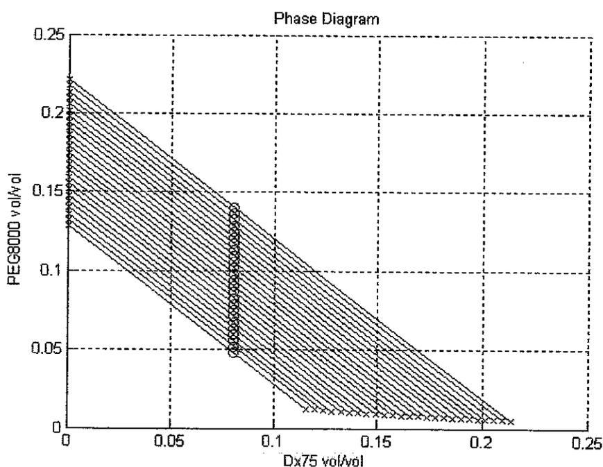
**Figure 14:** Phase Diagram for an ATPES of Water + PEG8000 + Dextran 75 + Human Hemoglobin at 23 °C after adjustment of scaling factors.
