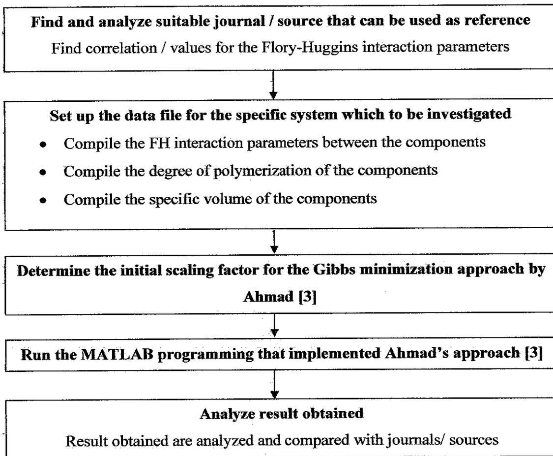
**Figure 5:** Steps in extending the approach by Ahmad [3] on predicting the LLE behavior based on an aqueous polymer system.
