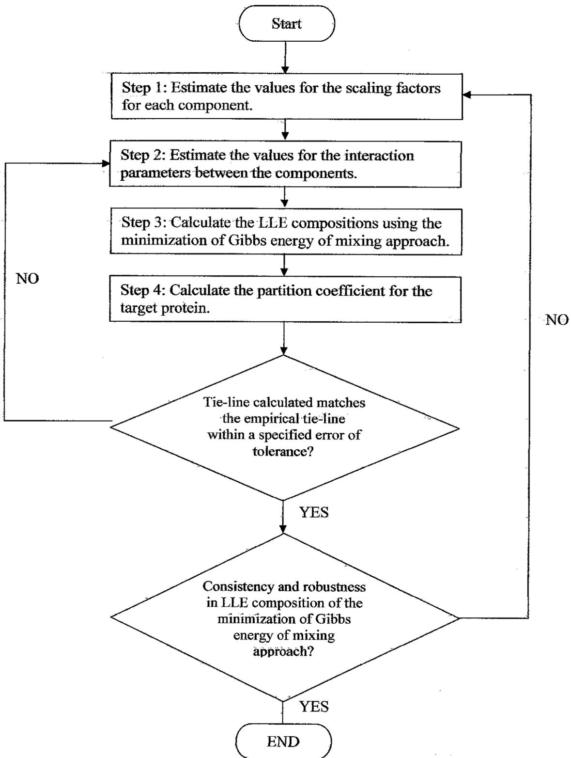
**Figure 6:** Manual partial enumeration strategy in determining the model parameters used in the ATPES modeling.
