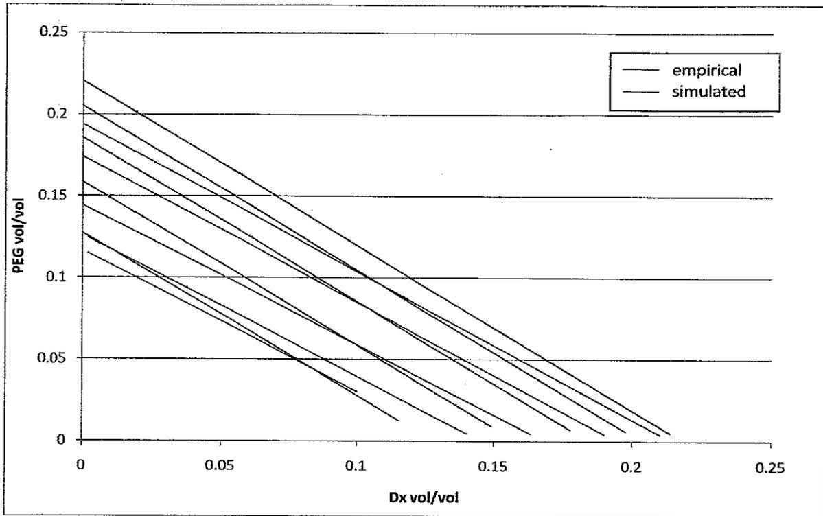
**Figure 19** : Comparison of phase diagram of water + PEG 8000 + Dx75 + human hemoglobin between empirical tie lines [30] and tie line simulated by modeling approach by Ahmad [3] on common plotting plane.
