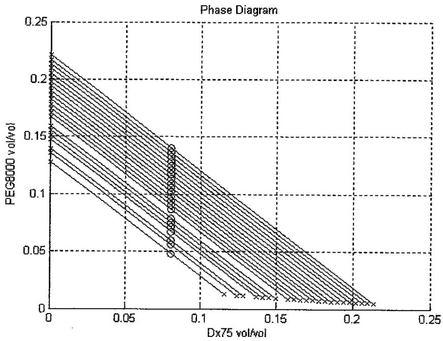
**Figure 18:** Phase Diagram for an ATPES of water + PEG8000 + Dextran 75 + lysozyme from chicken egg white at 23 °C
