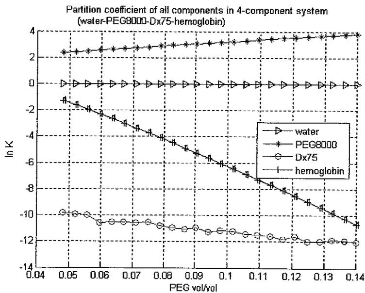
**Figure 13** : Partition coefficient of all components in 4-component ATPES of Water + PEG8000 + Dx75 + Human Hemoglobin at 23°C after adjustment of scaling factors.
