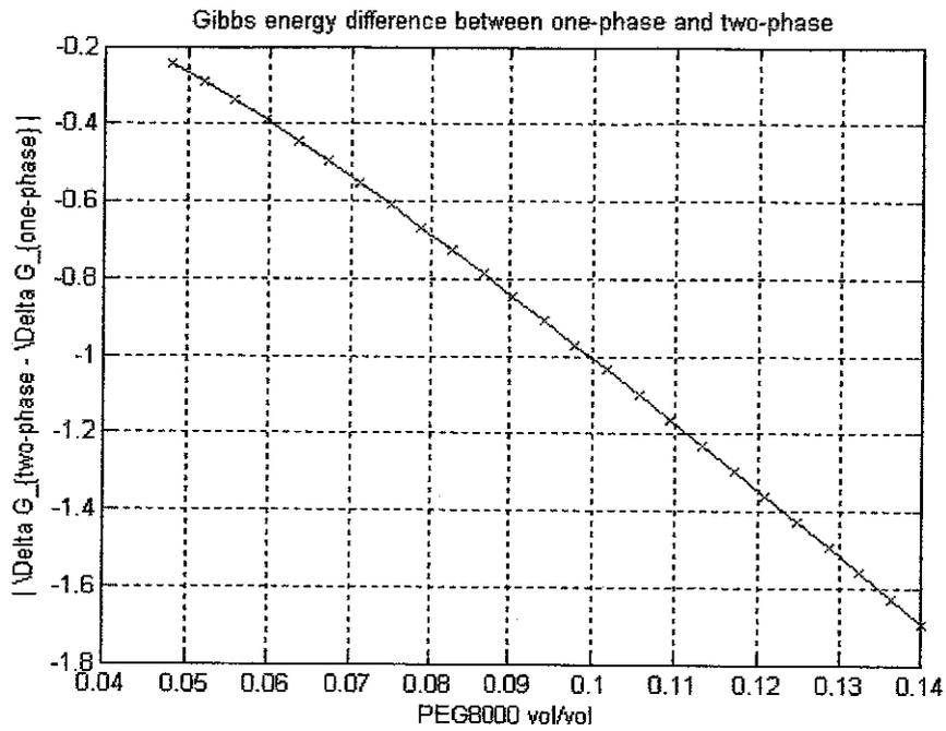
**Figure 12** : Gibbs energy difference between one-phase and two-phase for an ATPES of Water + PEG8000 + Dextran 75 + Human Hemoglobin at 23°C after adjustment of scaling factors.
