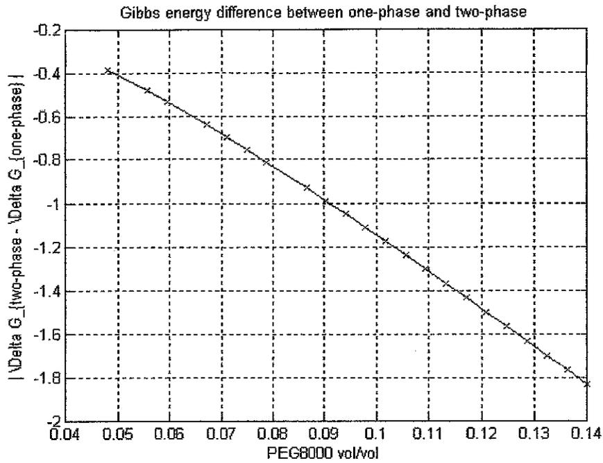
**Figure 16:** Gibbs Energy Difference Between one-phase and two-phase for an ATPES of Water + PEG8000 + Dextran 75 + lysozyme from chicken egg white (at 23°C)
