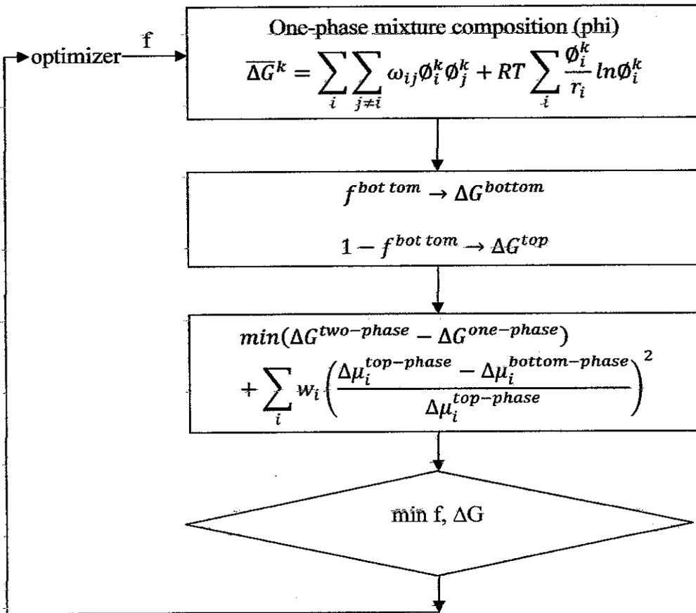
Figure 7: Algorithm of the MATLAB solver [3].
