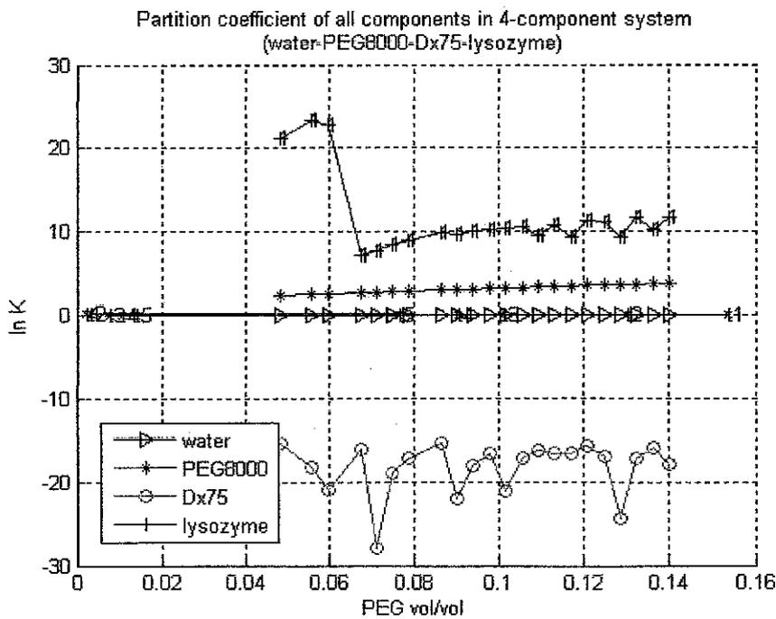
**Figure 17:** Partition coefficients in 4-component ATPES system of water + PEG8000 + Dextran 75 + lysozyme from chicken egg white at 23°C.
