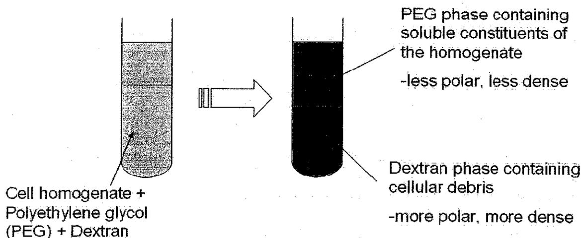
**Figure 1:** Aqueous two phase polymer system
