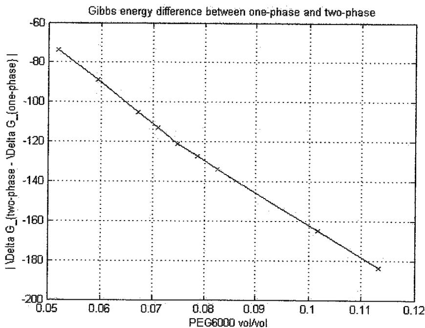
**Figure 9:** Gibbs Energy Difference Between one-phase and two-phase for an ATPES of Water + PEG 8000 + Dextran 75 + Human Hemoglobin at 23°C produced before adjustment of scaling factors.
