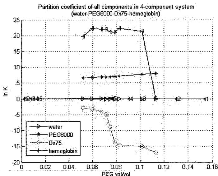
**Figure 10:** Partition coefficients in 4-component ATPES system of water + PEG8000 + Dx75 + human hemoglobin before adjustment of scaling factors.
