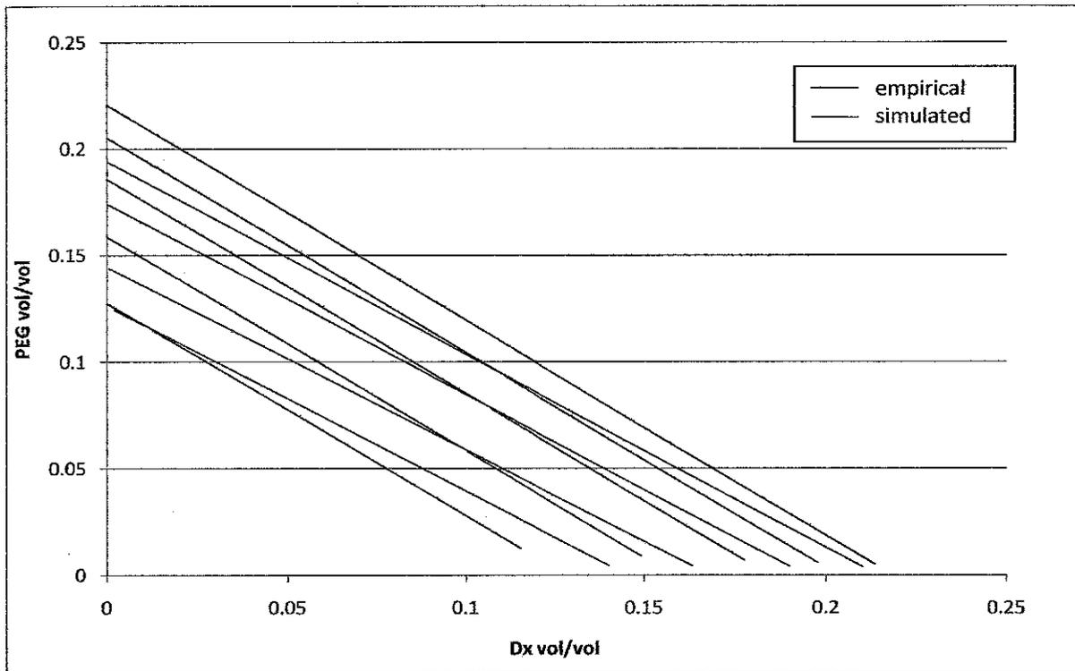
**Figure 20** : Comparison of phase diagram of water + PEG 8000 + Dx75 + lysozyme from chicken egg white between empirical tie lines [30] and tie line simulated by modeling approach by Ahmad [3] on common plotting plane.
