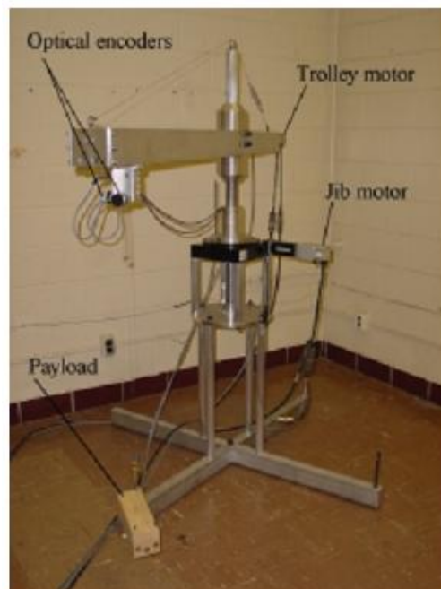
Figure 4.4: An experimental scale model of a tower crane.
