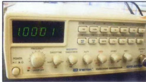
Figure 6 : Instek GFG-8250A Function Generator 5MHz
