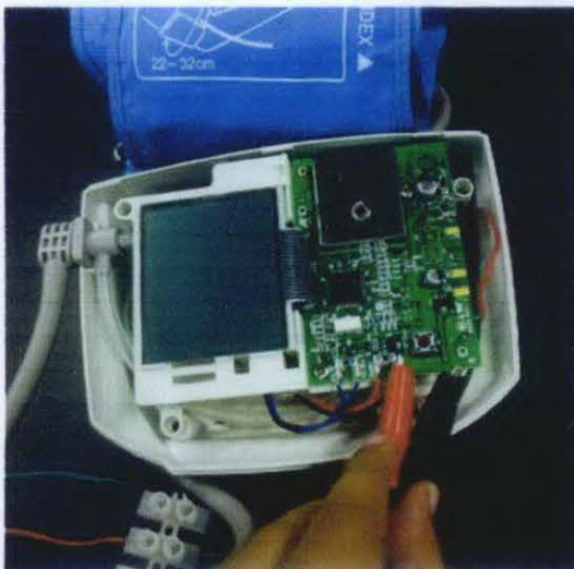
Figure17. Two open circuit wires
