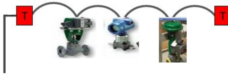
Figure 6 Daisy Chain Topology
