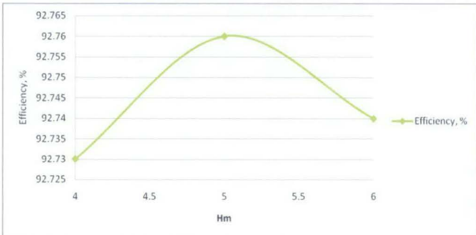
Figure 24 The Efficiency versus H_m of the Double Slot Linear Permanent Magnet Motor with Air-Cored.
