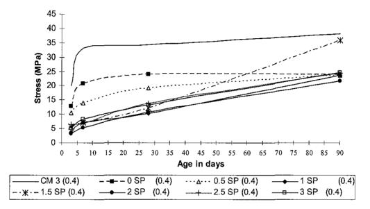
Figure 16: Compressive strength results for 0.4 w/c.
