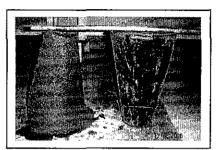
Figure 10: Slump test for 0SP Slump = 13mm ~ Low workability.
