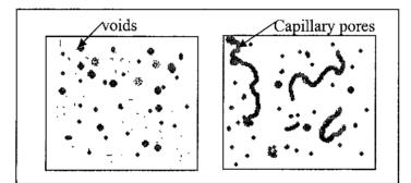
Figure 19: Comparison of pores distribution and connectivity between two same porous samples.
