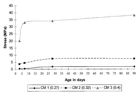
Figure 14: Compressive strength results for Control Mix.
