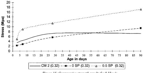
Figure 15: Compressive strength results for 0.32 w/c.
