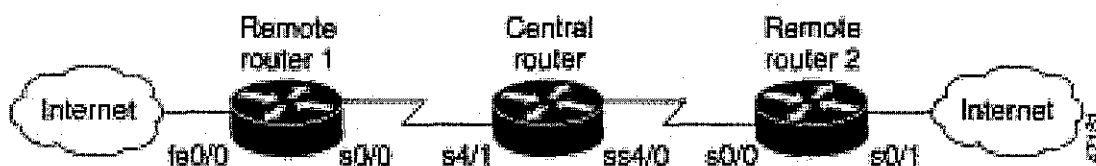
Figure 5: Sample Network Implementing Diffserv
