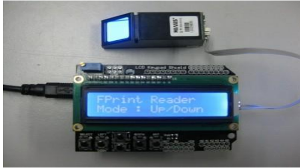
Figure 13: Fingerprint Module Interfaced with Arduino Uno
