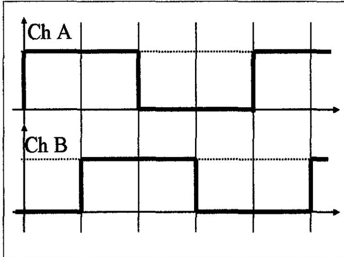
Figure 2: The channel waves of the mouse encoder
