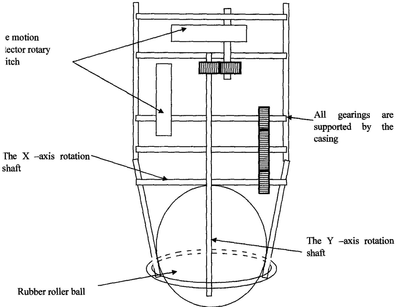
Figure 13: Pen Mouse design with mechanical gearing to move the encoder shaft for the photo sensitive to detect the waveform required for the computer to translate it in motion in x and y directions.
