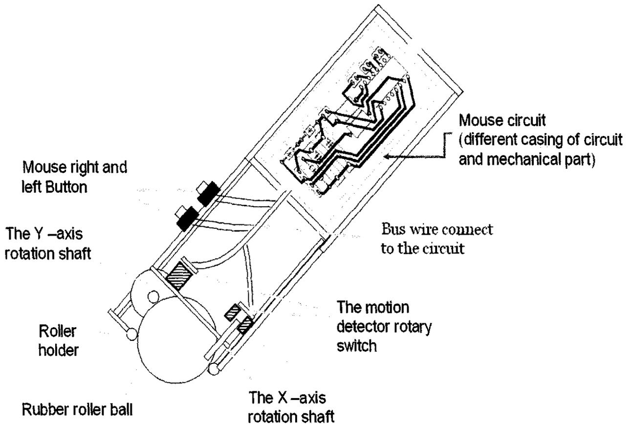
Figure 14: Improvement to Pen Mouse design 3 with roller holder. The project mouse model currently refers to this design. Due to its practical position of the shaft.
