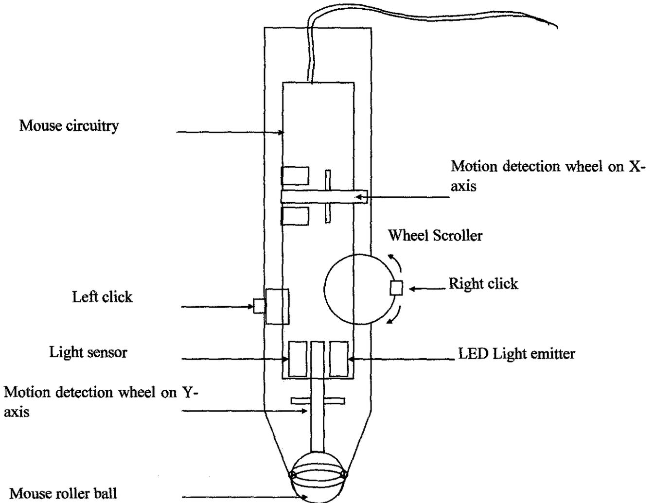
Figure 12: Pen mouse design 1 has unpractical shaft position that allows the ball to move in only one axis. The design is not selected to construct the pen shape mouse.
