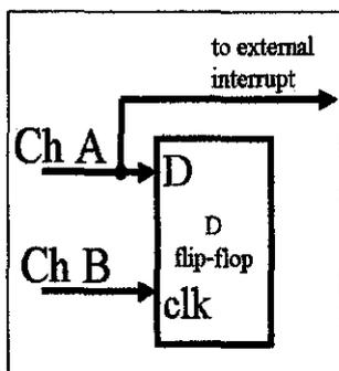
Figure 3: Flip flop for mouse encoder
