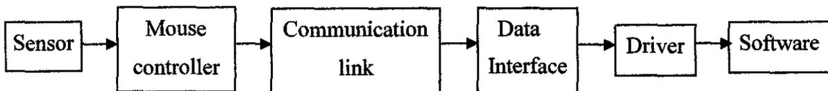
Figure 1: Typical mouse controlling system stages
