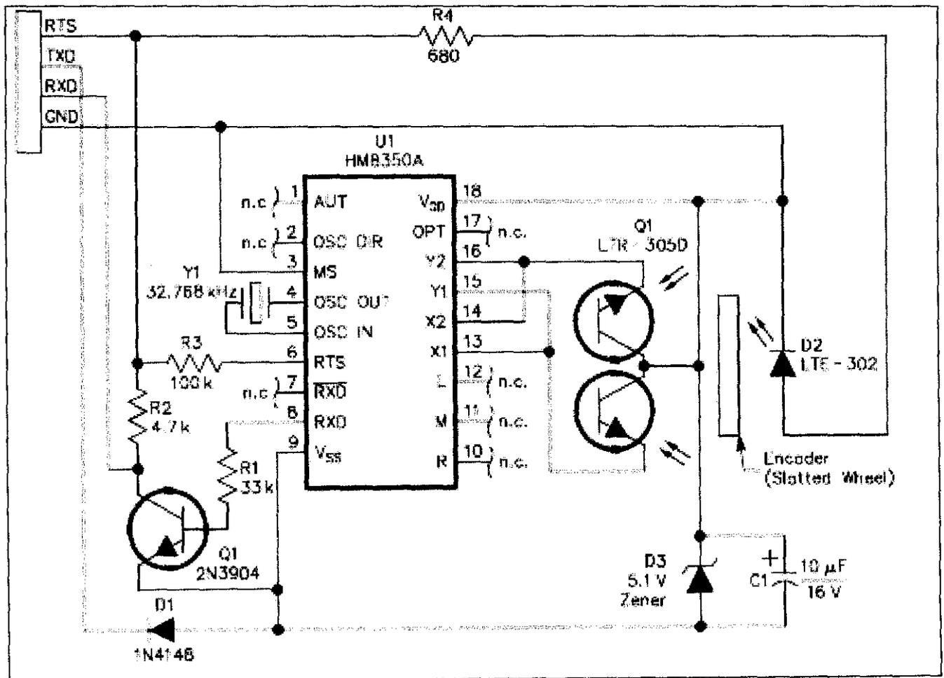
Figure 15: Schematic diagram of a conventional ball type mouse. The circuit consist of power input, input for X and Y axis motion signal, 3 button input (Left, Right and middle click), and three led source for generating the motion binary signal.
