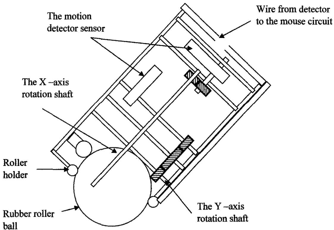
Figure 10: Pen Shape Mouse Design final drawing selection
