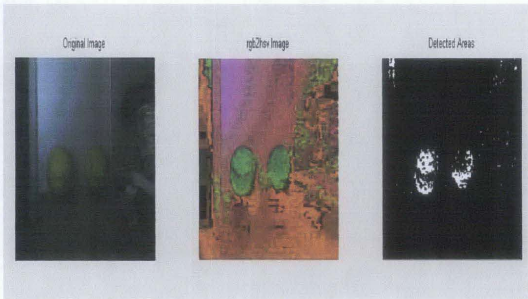
Figure 15: Real Time HSI Colour Detection Algorithm Output Image
