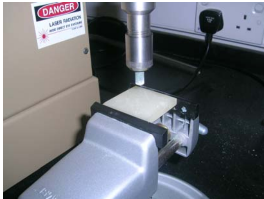
Figure 3.15 : Installing the specimen and wearaser to the machine
