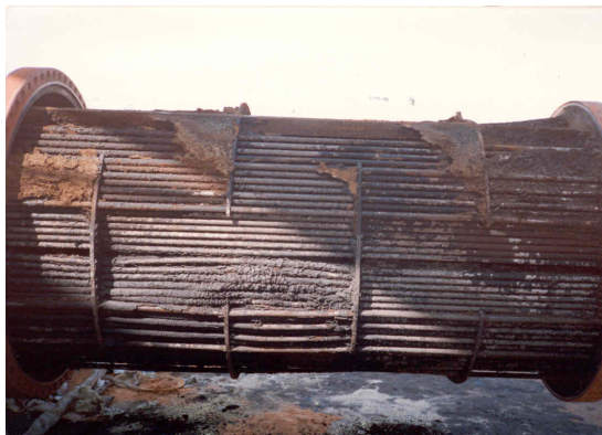
Figure 4: Fouling of heat exchanger caused by asphaltene precipitation
