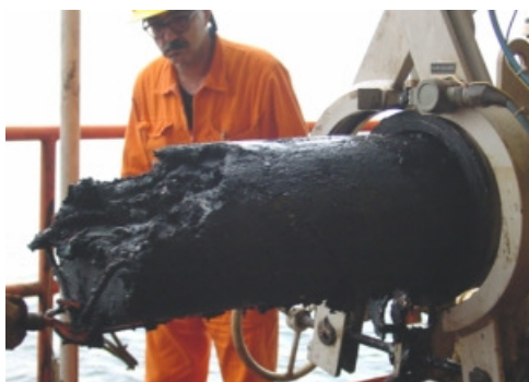
Figure 3: A crude oil pipeline blocked by asphaltenes and waxes.
