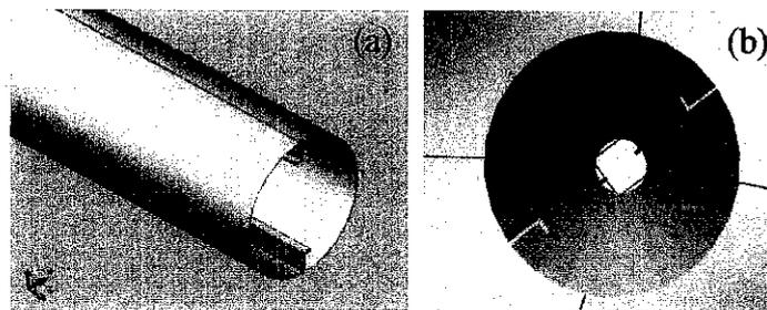
Figure 12 Drum granulator designed with scoops. (a) Isometric view (b) Front view
