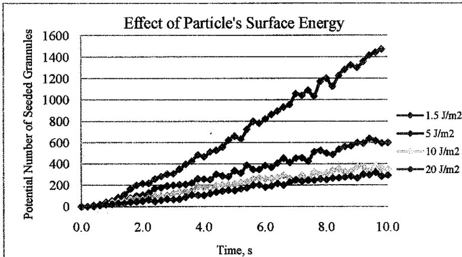
Figure 15 Potential seeded granules at different surface energy.
