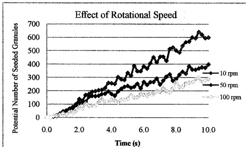
Figure 14 Potential seeded granules at different drum rotational speed, using model granulator without scoops.
