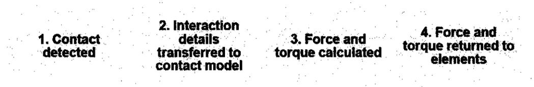
Figure 7 Methodology used by EDEM during simulation.
