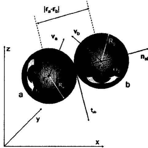
Figure 3 Coordinate system used to describe collision model in DEM (Deen *et al.*, 2007).
