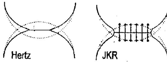
Figure 4 Illustration of the difference between two most used particle contact models (Contact Mechanics, 2012)
