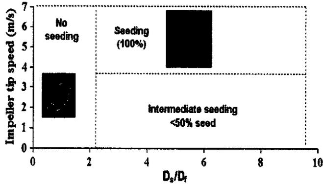
Figure 2 Regime map presented for production of seeded granule structure in Cyclomix granulator (Rahmanian *et al.*, 2011)
