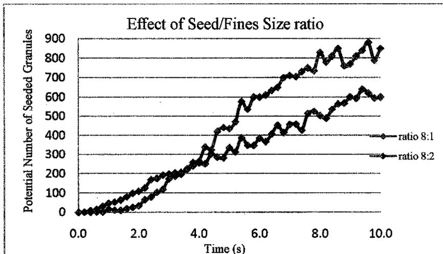
Figure 16 Potential seeded granules at different seed/fines size ratio.
