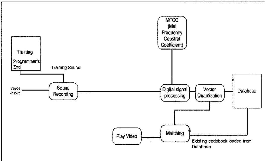
*Figure 3.1.3-1: Data Flow Diagram*
