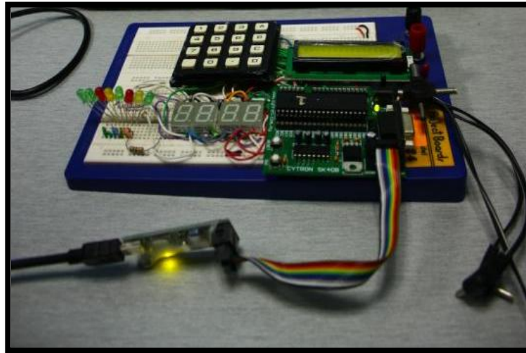
Figure 21: The circuit with LEDs, Keypad, LCD and the debugger connected
