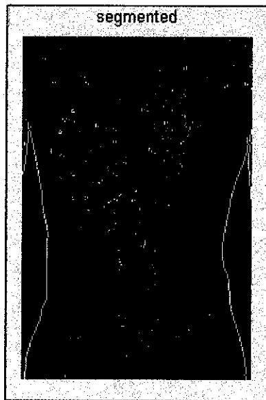
Figure 3.3: Result of image after the segmentation of scaliness using Sobel edge detection and thresholding techniques.
