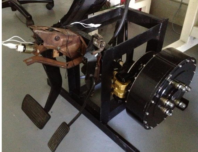
Figure 9: Complete brake pedal assembly with BLDC motor
