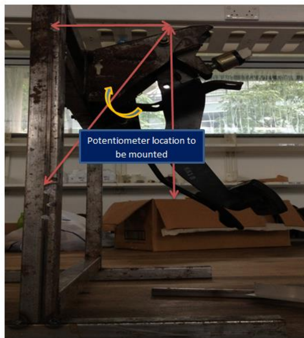
Figure 10: Illustration to design and calculate the position for linear sensor
