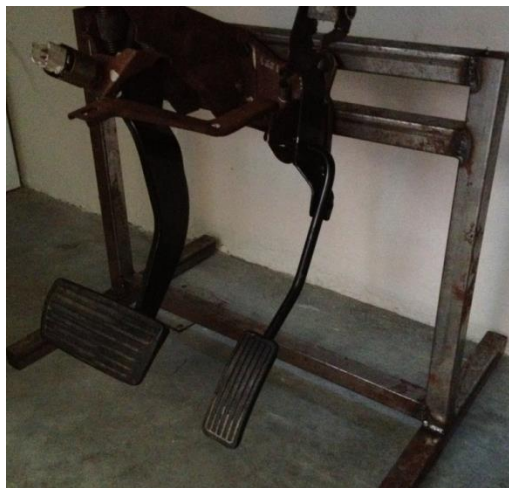
Figure 8: Pedal brake assembly on bracket stand
