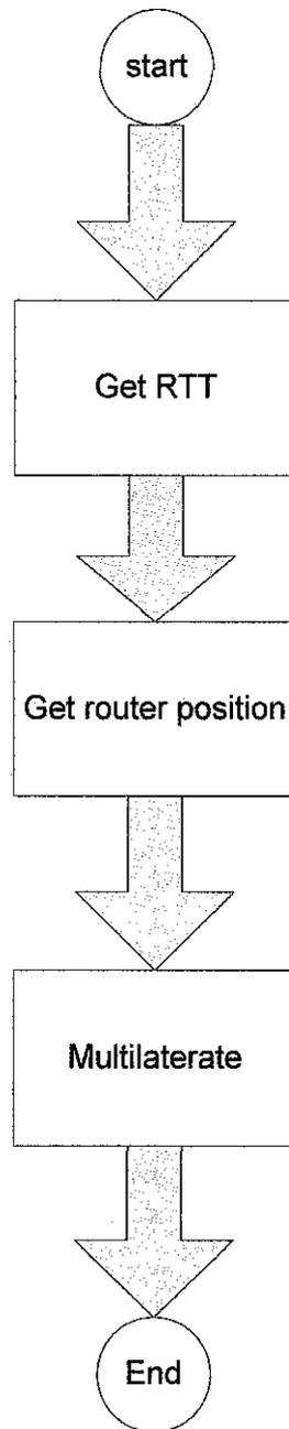
**Figure 20 - calculate position flowchart**
