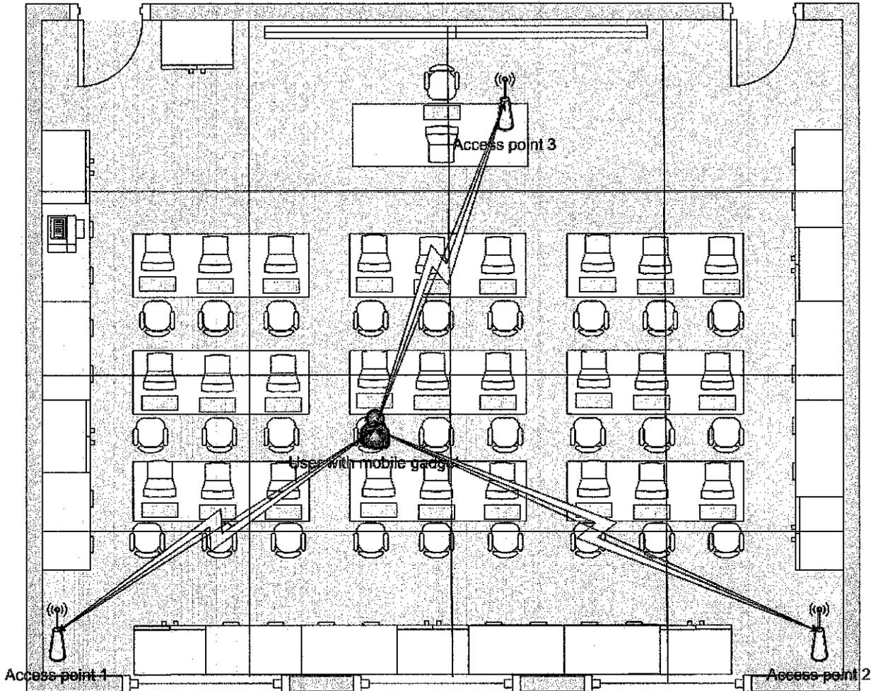
**Figure 13 - Multilateration positioning Experiment**
