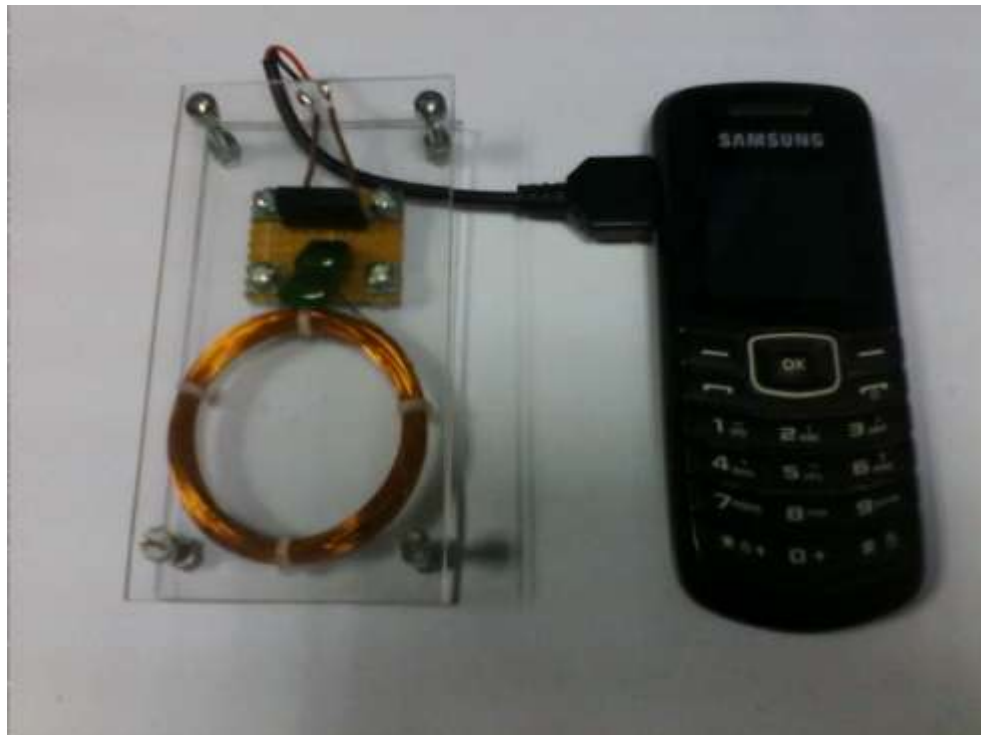
Figure 29 : The receiver prototype connected to cellphone with 3.7V Li-ion battery.
