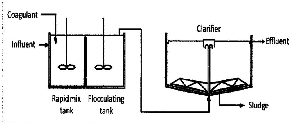
Figure 2.1: Clarification system incorporating coagulation and flocculation
