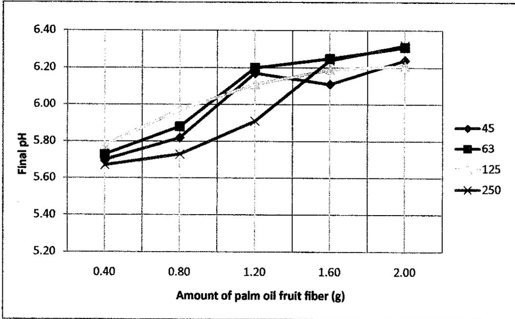
Figure 5.0 Final pH versus amount of palm oil fruit fiber for different particle size
