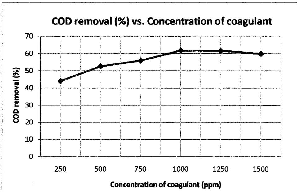
Figure 4.3 COD removal (%) versus different concentration of coagulant
