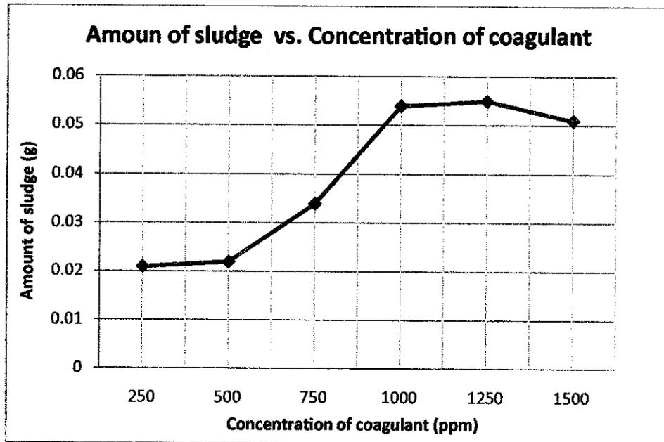
**Figure 4.4** Amount of sludge formed versus different concentration of coagulant
