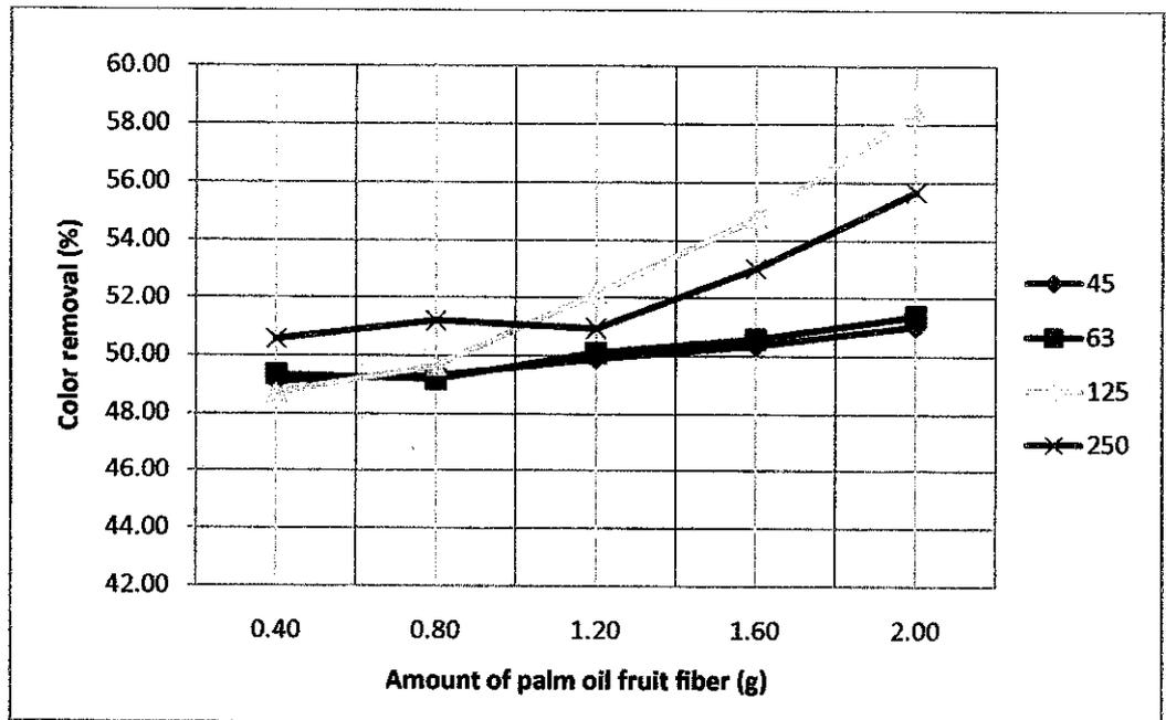
Figure 5.1 Color removal versus amount of palm oil fruit fiber for different particle size
