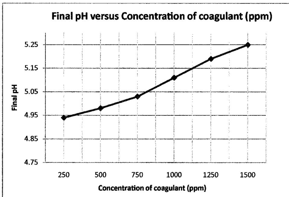
**Figure 4.1 Final pH versus different concentration of coagulant**
