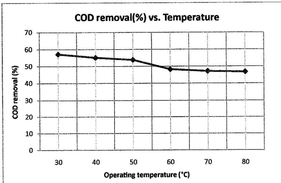
Figure 4.9 COD removals (%) versus different initial temperature
