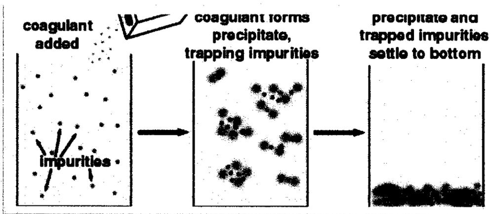
Figure 2.2: Coagulation and flocculation mechanism
