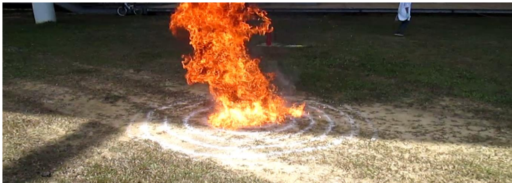
Figure 9: Experiment 1 (2 cm fuel thickness)
