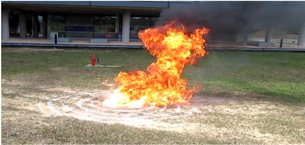
Figure 11: Experiment 3 (4 cm fuel thickness)
