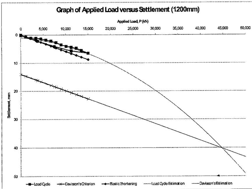
**Graph 4.9: Graph of Applied Load versus Settlement (1200mm Pile)**
