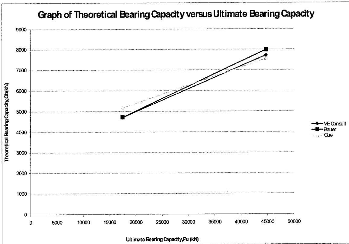
**Graph 4.10: Graph of Theoretical Bearing Capacity versus Ultimate Bearing Capacity**
