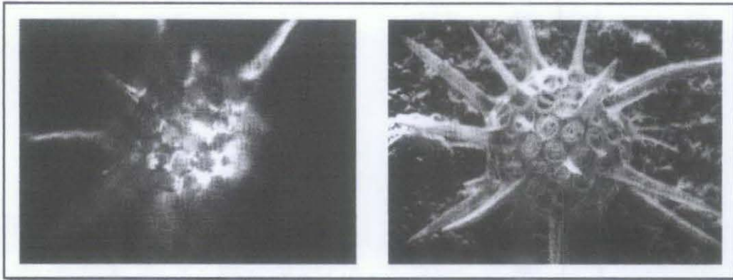
Figure 2.4: Difference in result between Optical Microscope (left) and Scanning Electron Microscope (right) [12] (taken from Goldstein et al. 1992)
