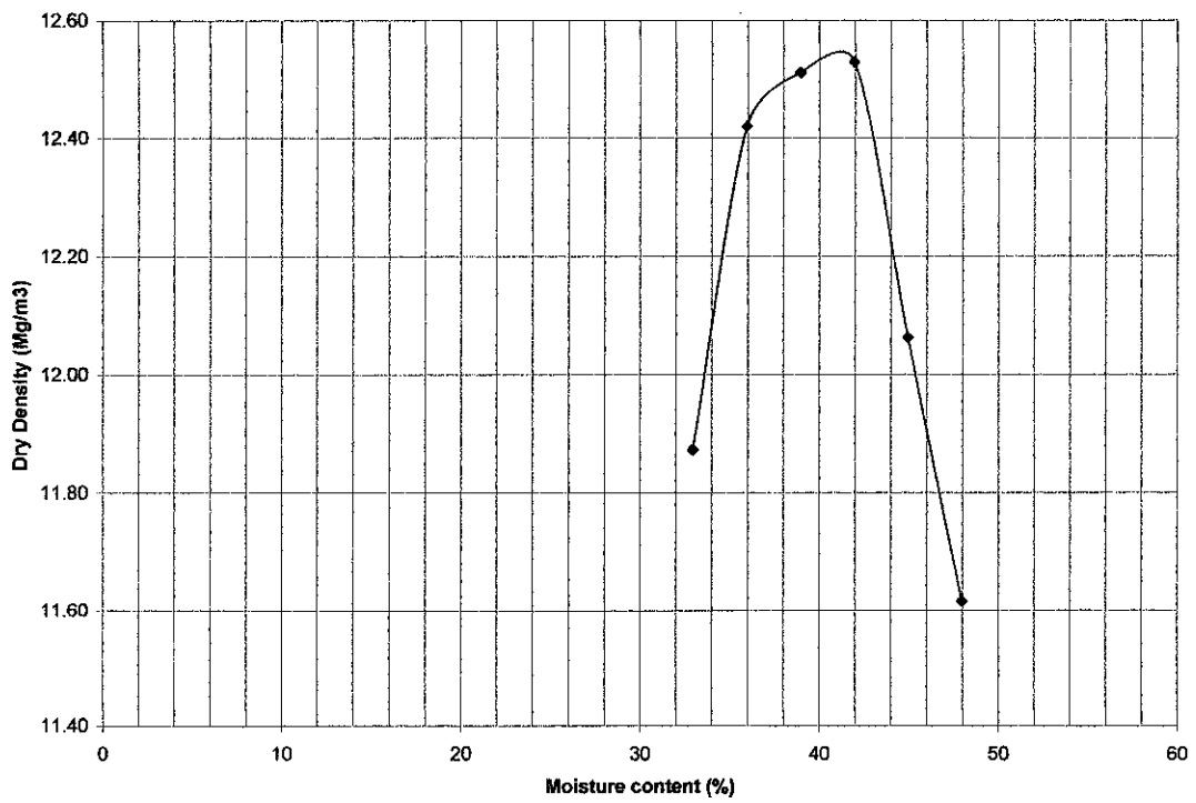
Dry density (Mg/m 3 ) vs moisture content (%) for 36% Rha
