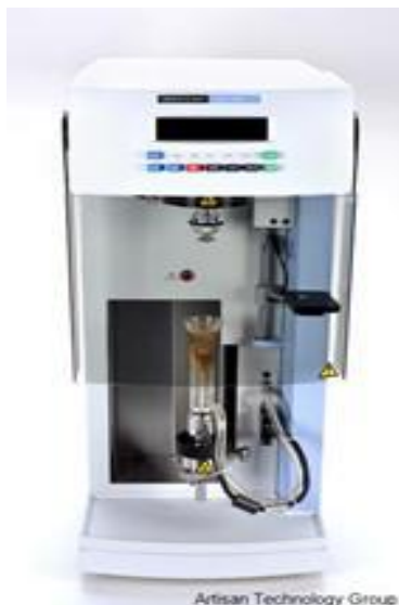
Figure 5: Thermal Gravimetric Analyzer Perkin Elmer Pyris 1
