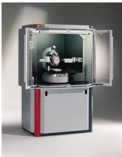
Figure 6: X-Ray Diffraction Bruker-AXS D8 Advance
