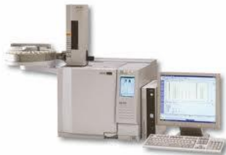
Figure 11: Shimadzu GC-2010 used for liquid phase analysis
