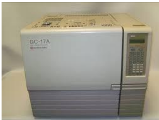
Figure 10: Shimadzu GC-17A used for gas phase analysis
