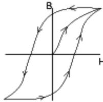
**Figure 2.5 Typical B-H Curve**
