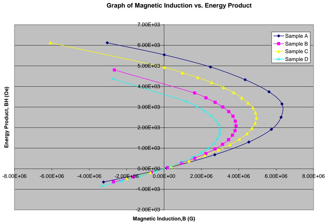
**Figure 4.5: Graph of B versus BH for Sample A, B, C, and D**
