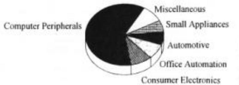
**Figure 2.3: Breakdown of applications of bonded NdFeB [12]**
