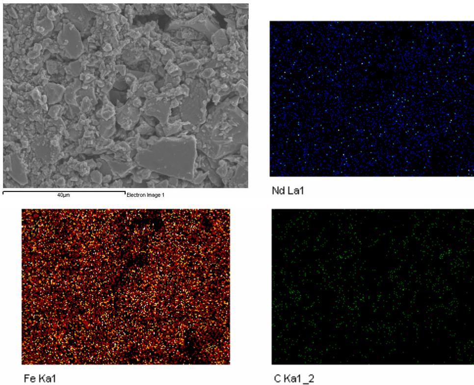
**Figure 4.4: EDX mapping shows the element distribution in the sample**
