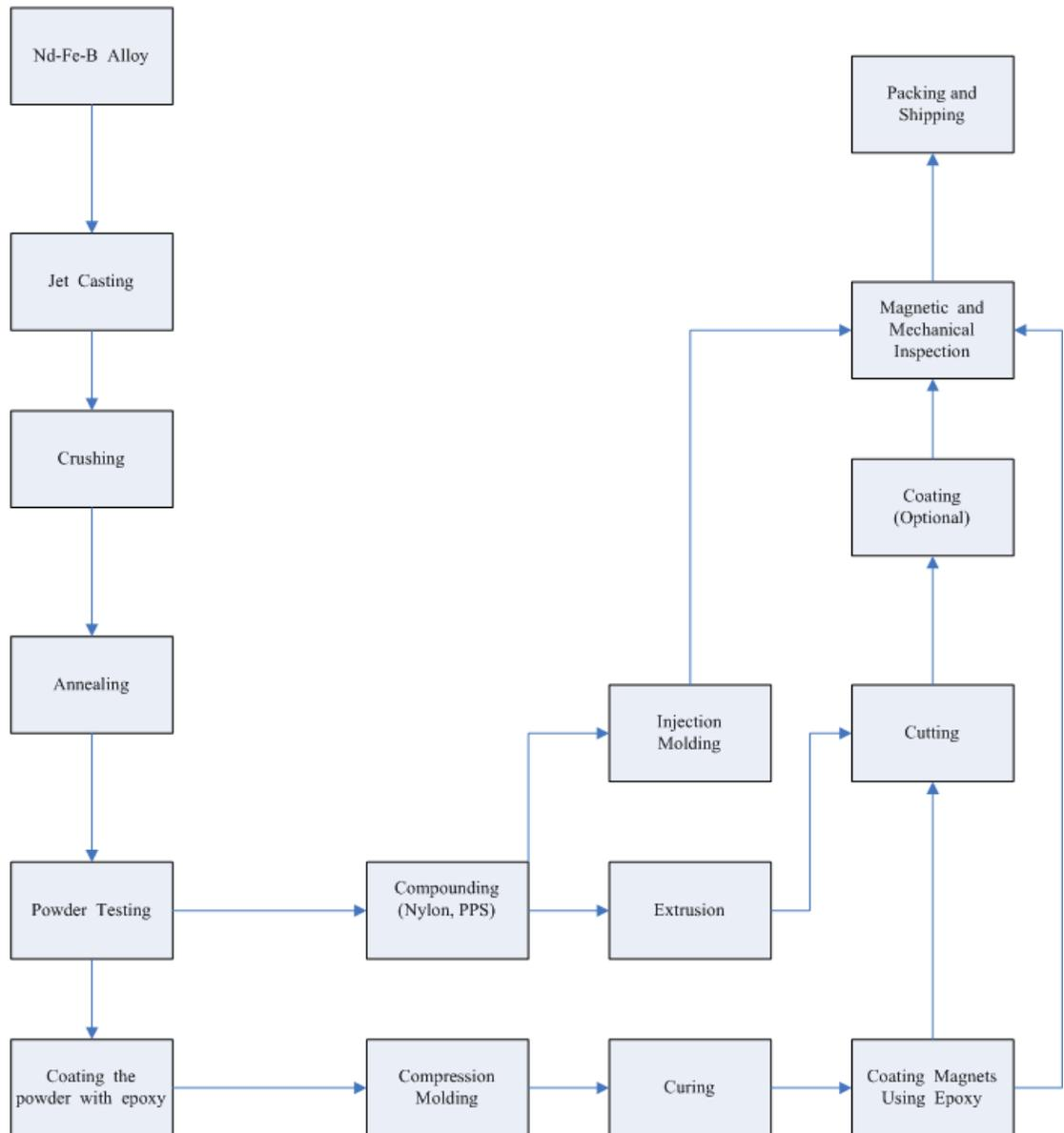
**Figure 2.2: Typical Manufacturing Process of Bonded NdFeB Magnet [16].**
