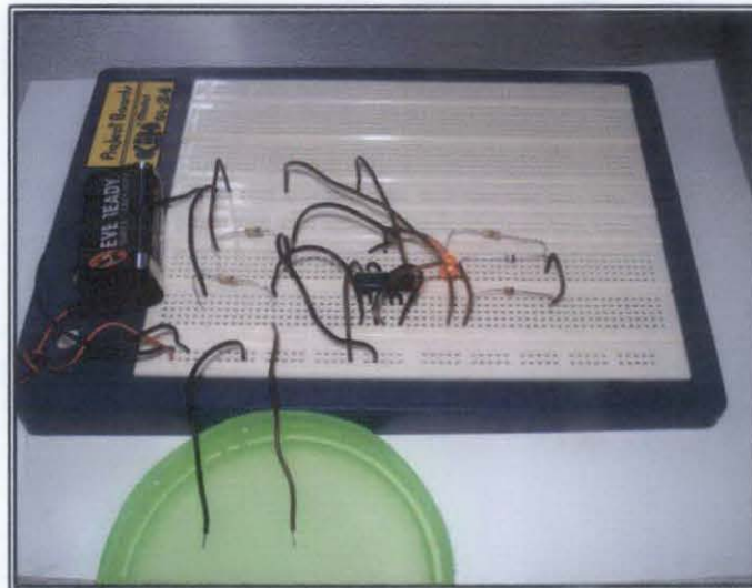
Figure 17: Constructed water level sensor
