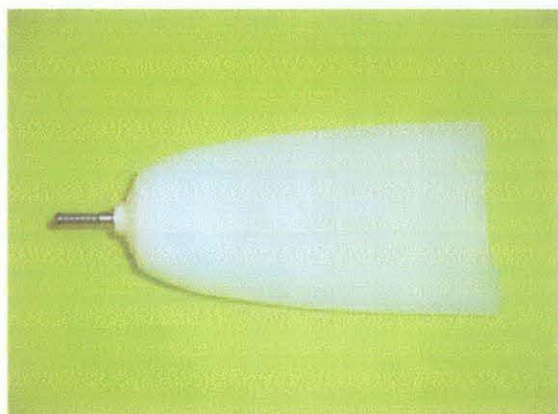
Figure 40: The final plastic part of the prosthetic leg socket after rapid tooling process.
