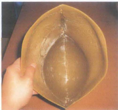
Figure 37: Top view of the completed rapid prototype prosthetic leg socket after combined with the superglue.
