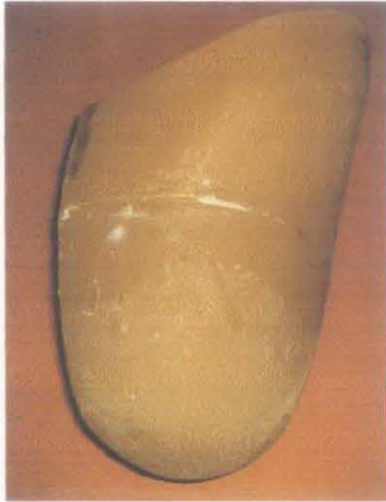
Figure 36: Side view of the completed rapid prototype prosthetic leg socket after combined with the superglue.
