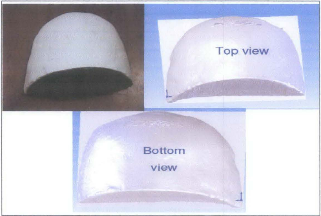
Figure 31: part 1 of the amputee stump with the solid modeling in Unigraphics.
