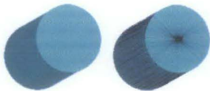
Figure 24: Comparison of good STL and bad STL file format
