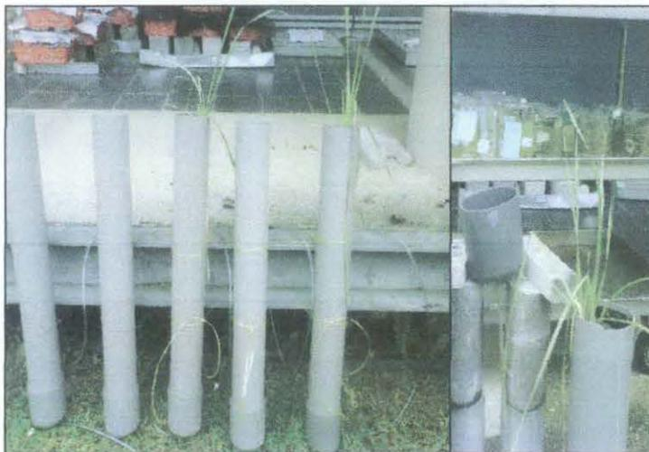
Figure 22: The Physical Model of Bioretention in Laboratory
