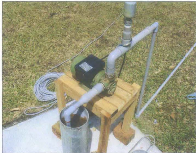
Figure D-3. Automatic Centrifugal pump
