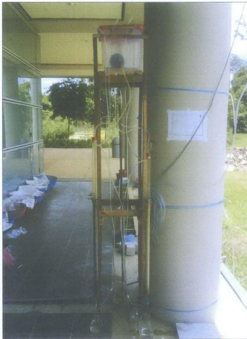
Figure D-4. Set up for Direct Groundwater Filtration Experiment
