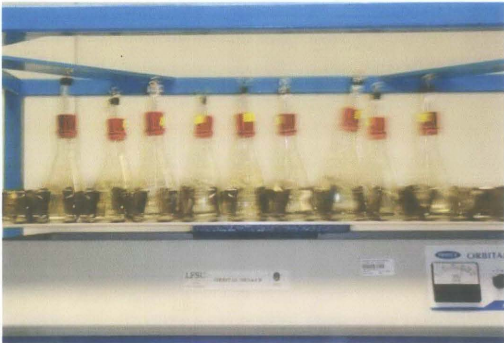
Figure D-2. Experiment Procedure in Adsorption and Catalytic Effect of Sand and Carbonaceous Shale of Ferrous Iron
