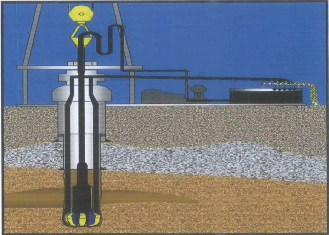
Figure 4.2: Hydraulics Optimization Circulation system.
