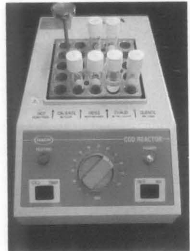
Figure 28 : Heat the sampels with 150°C about 2 hr
