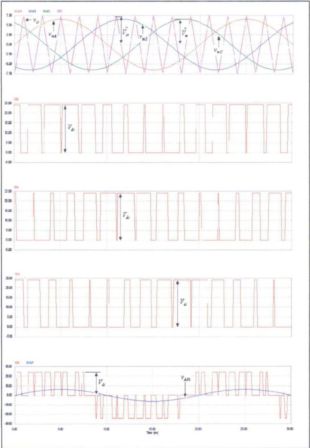
Figure 24: Sinusoidal Pulse Width Modulation signal
