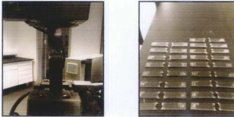
Figure 4.10: Fractured samples after tensile test
