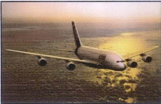
(a): The Airbus A380 has about 26 tons of hybrid composite in each airconf
