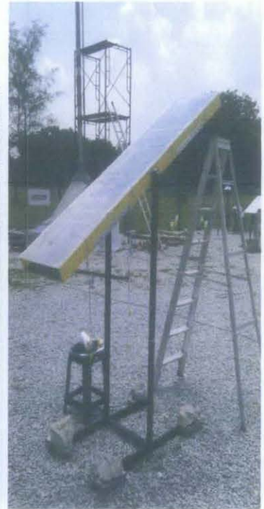
Figure 3.9 2m wall channel at 30°
