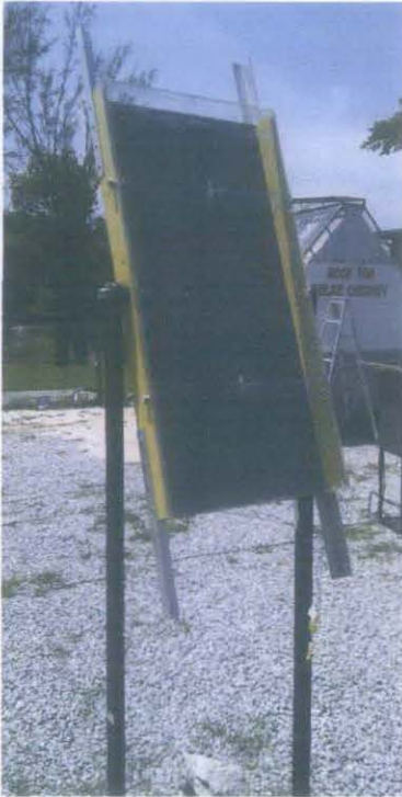
Figure 3.7 1m wall channel at 30°
