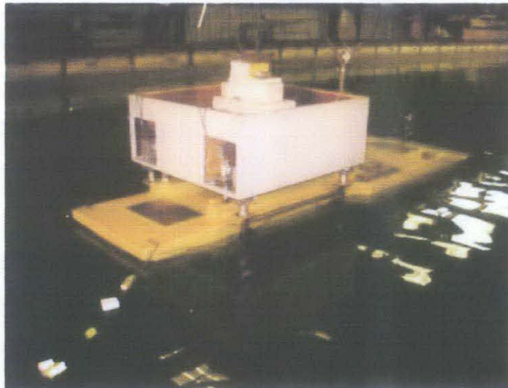
Figure 10: Float-over model using I-650
