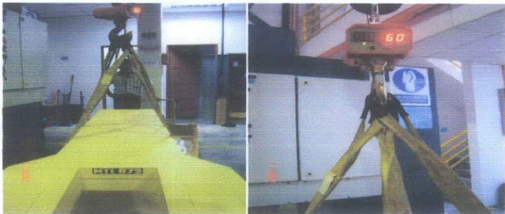
Figure 24: Mass of barge = 60kg
