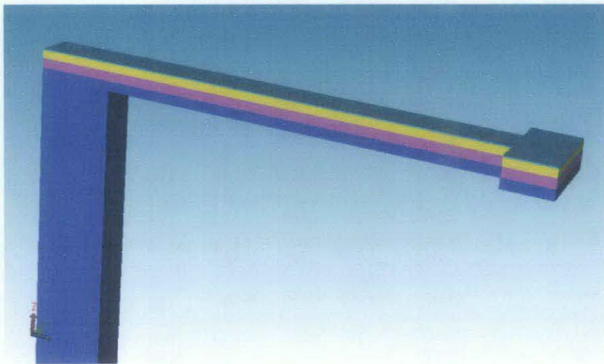
Figure 10: 3D Model Showing Layers of Cantilever Beam
