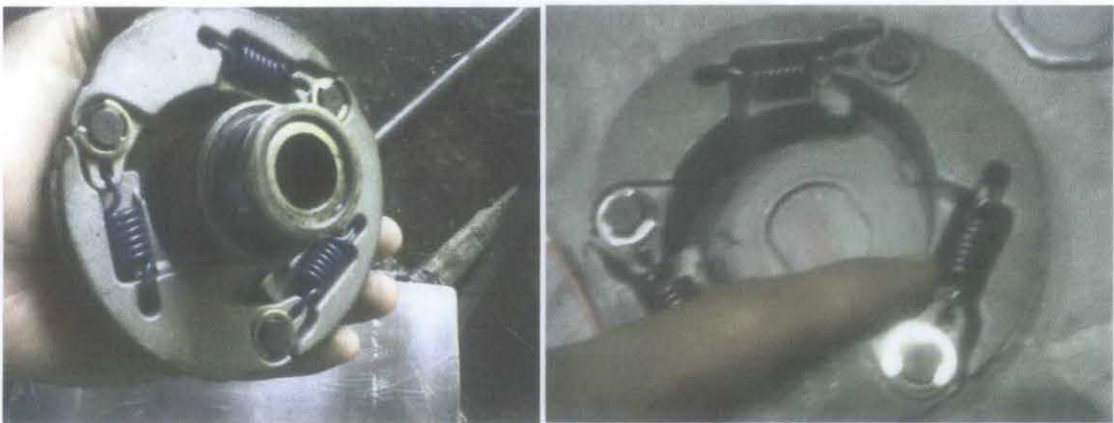
Figure 4.4 (a) and 4.4(b): spring clutch before and after modification
