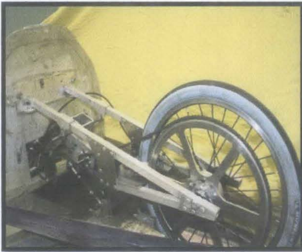
Figure 2.6.1 Direct transmission of the car
