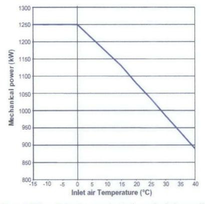
Figure 3: Effect of inlet air temperature to the mechanical power [9]
