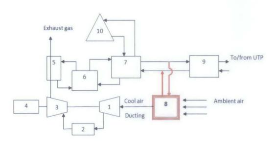
1-compressor; 2-combustor; 3-turbine; 4-generator; 5-HRGS; 6-boiler; 7-steam absorption chiller; 8-air cooler; 9-heat exchanger; 10-cooling tower
