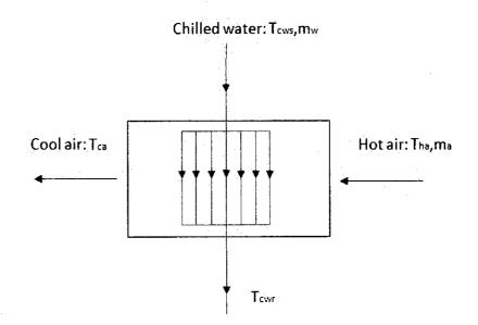
Figure 9: System diagram
