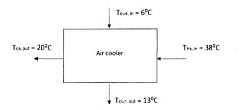
Figure 11: inlet and outlet temperature
