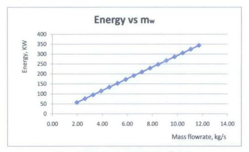
Figure 15: Energy versus water mass flowrate
