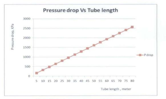
Figure 16: Graph pressure drop versus tube length
