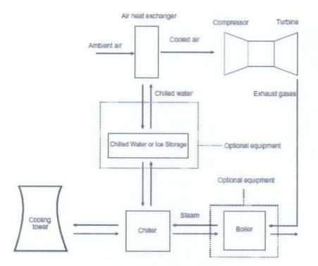
Figure 4: Generic inlet air cooling system [10]
