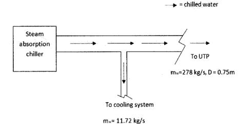
Figure 10: distribution of chilled water mass flowrate
