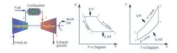
Figure 1: PV and TS diagram of a Brayton cycle mapped to actual of a gas turbine engine [15]
