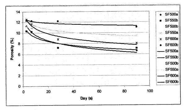
Figure 4.4: Porosity of concrete sample
