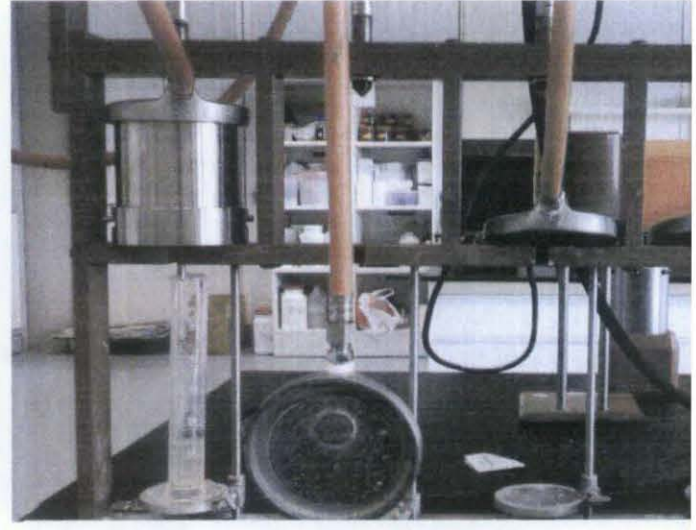
Figure 13: The Low Pressure Low Temperature (LPLT) alternative to the Permeability Plugging Test to measure Filtrate Loss
