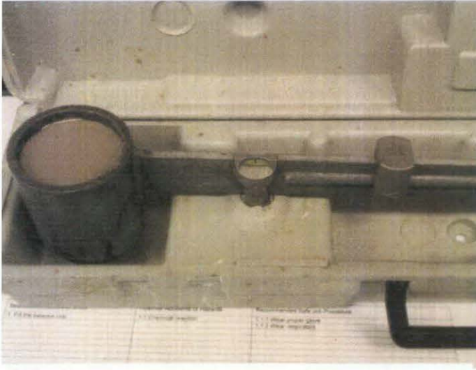
Figure 12: Mud scale used to measure mud weight in pound per gallon
