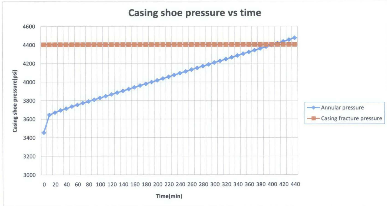
Figure 12: Casing shoe pressure versus time for 20 md gas formation
