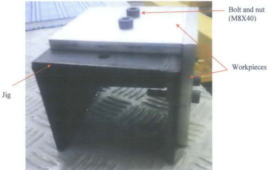
Figure 4.7 – The arrangement of jig and plate
