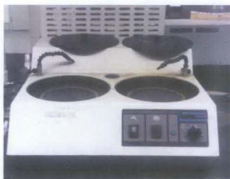
Figure A-3.3 – Grinding and polishing Machine
