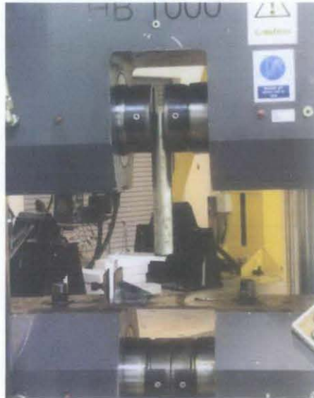
Figure 4.11 – Peel-Off Test setup
