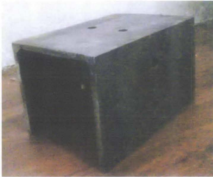
Figure 4.2 – The jig for 90 degrees corner plate
