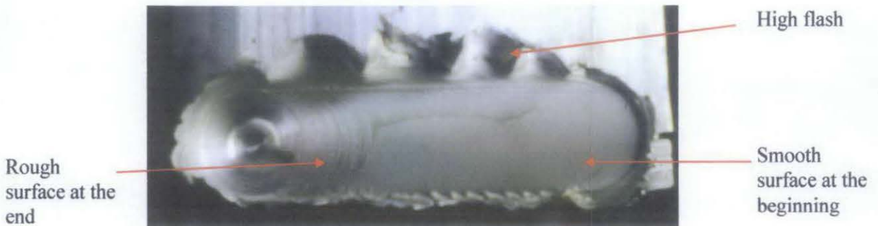
Figure 4.8 – Sample (1000 rpm, 8mm/min)
