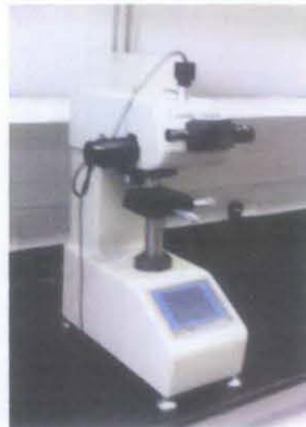
Figure 4.18 – Vickers Microhardness test
